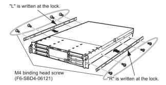
Left and right inner rails are different. Check the letter at the lock part for correct installation.
